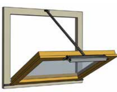
Bottom hung window / Top hung window inward opening; Actuator top middle on sash at the main closing edge
