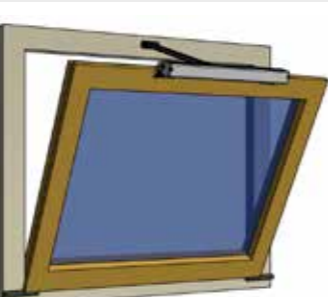
Bottom hung window / Top hung window inward opening; Actuator top middle on sash at the main closing edge
