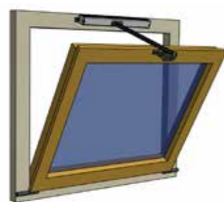
Bottom hung window / Top hung window inward opening; Actuator top / bottom middle on frame at the main closing edge
